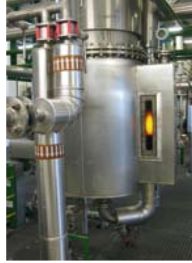
Measurement with guided radar: Levelflex interface in the bypass
